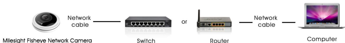
Figure 2-1-2 Connect via a switch or a Router
