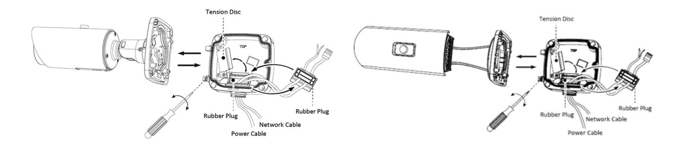
Step4: Connect the front and rear cover on the left side so that the clamshell structure is formed. In the end, close the two covers and fix the screw to finish the installation.
