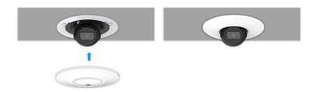
Step 6: Connect the cable and insert the camera with the mounting adaptor to the ceiling;
