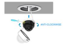
Step 11: Loosen the clamp screw on the camera, adjust the lens to the correct direction and tighten the clamp screw;
