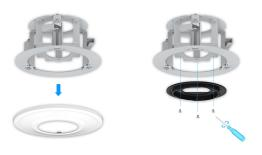
**Step 4:** Rotate the camera to the mounting bracket and make sure it is positioned correctly;
