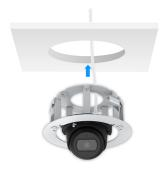
Step 8: Loosen the clamp screw on the camera, adjust the lens to the correct direction and then tighten the clamp screw;
